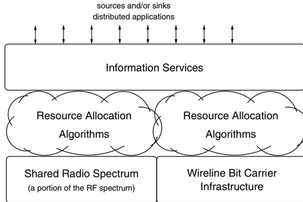
**Figure 1.1 A conceptual view of distributed applications utilizing wireline and wireless networks. Wireless networking is concerned with algorithms for resource allocation between devices sharing a portion of the radio spectrum. On the other hand, in wireline networks the resource allocation algorithms are concerned with sharing the fixed resources of a bit transport infrastructure.**
