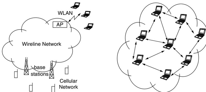
**Figure 1.3 The left panel shows some access networks (a cellular telephony network, and a wireless local area network (WLAN), where the access is via an AP (access point)), and the right panel shows a mesh wireless network of portable computers.**
